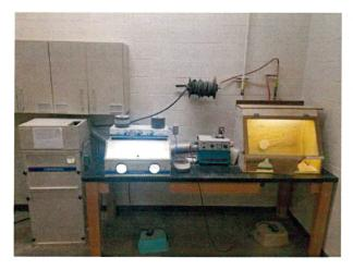
The current air chamber is not sealed and leaks dust and other hazardous fumes into the lab area. An updated dust collection system and the  $2 \times 3 \times 2$ -foot air chamber will protect Survey paleontologists, volunteers, and guests from exposure to potentially harmful dust.
