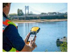
NDGS geologists currently use commercial grade Garmin GPS units for logging the location of fossil and mineral localities with horizontal accuracy of around 3 meters. The Trimble TDC150 is a differential grade GNSS receiver capable of centimeter-scale accuracy, necessary for resolving tight sampling intervals, closely spaced fossils, or high-precision drone surveys. Centimeter accuracy.
