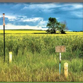
Groundwater monitoring wells (yellow pipes) are located across the state.
