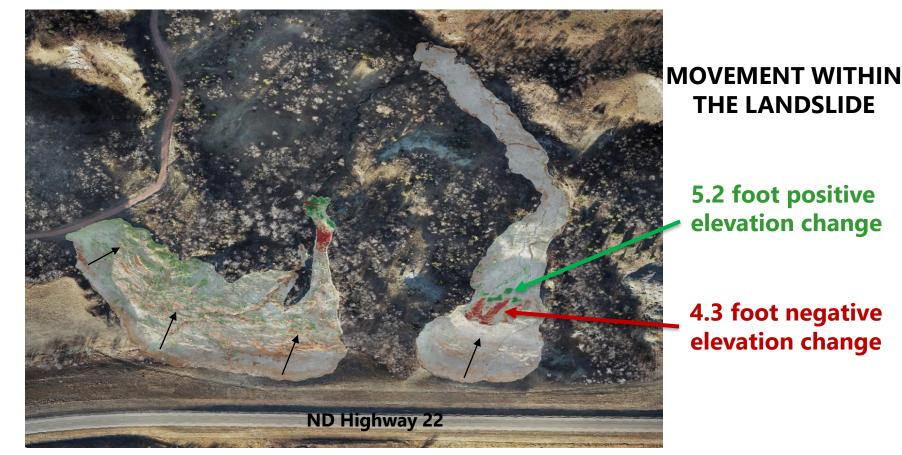
The highlighted areas are comparative 3D models created from 1,350 photos from our October 8, 2019 drone flight and 1,500 drone photos from our November 24, 2020 flight. Arrows point in the direction of slope movement. We estimated 420,000 tons of slide material.
