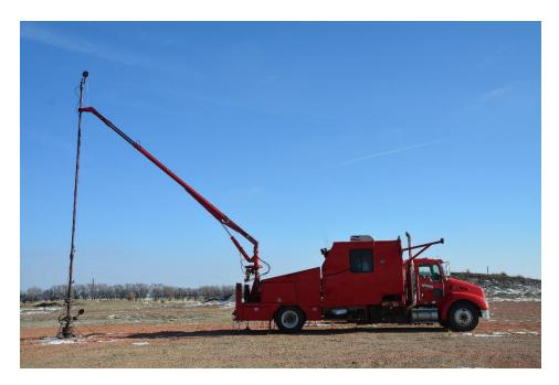
Left: Black dots are wells we have temperature logged, green dots are wells that were temperature logged January 4-7, 2021, and the gray dots are TA'd wells that are potential candidates for logging. Right: Temperature probe being dropped into a TA'd well via a slick line truck.
