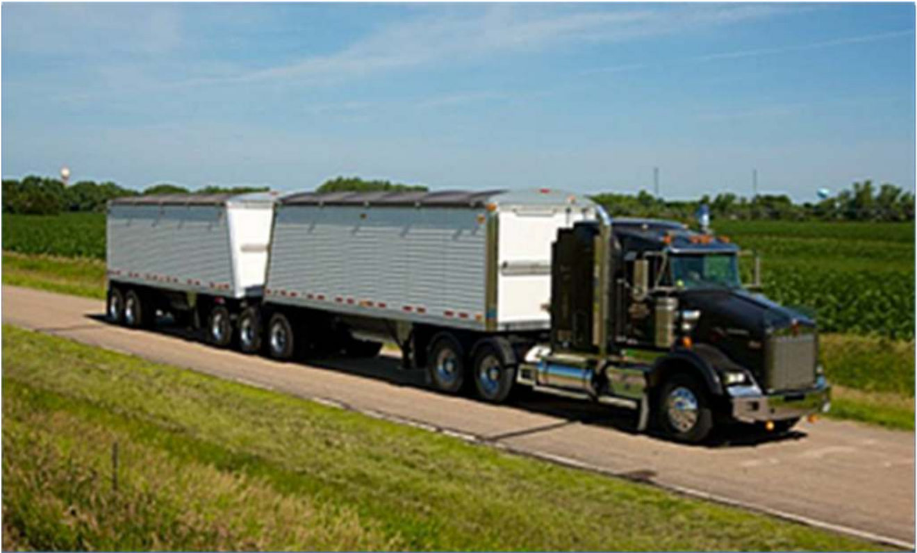
Figure 4. Canadian 8-Axle B Train with Fifth Wheel Tridem Axle
