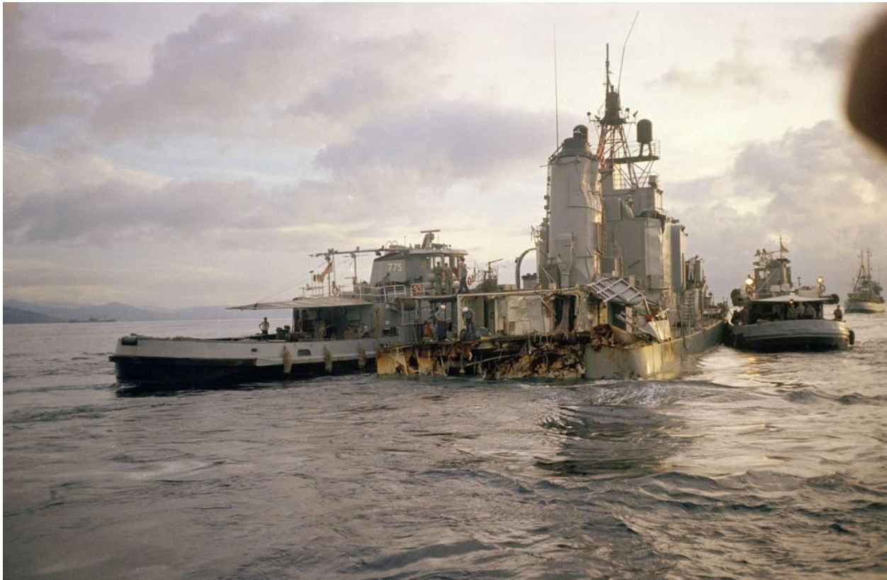
Sailors inspect damage to the U.S. Navy destroyer Frank E. Evans after it was cut in half in a collision with the light aircraft carrier Melbourne of the Royal Australian Navy in the South China Sea, 650 miles southwest of Manila, June 3, 1969. (AP)
