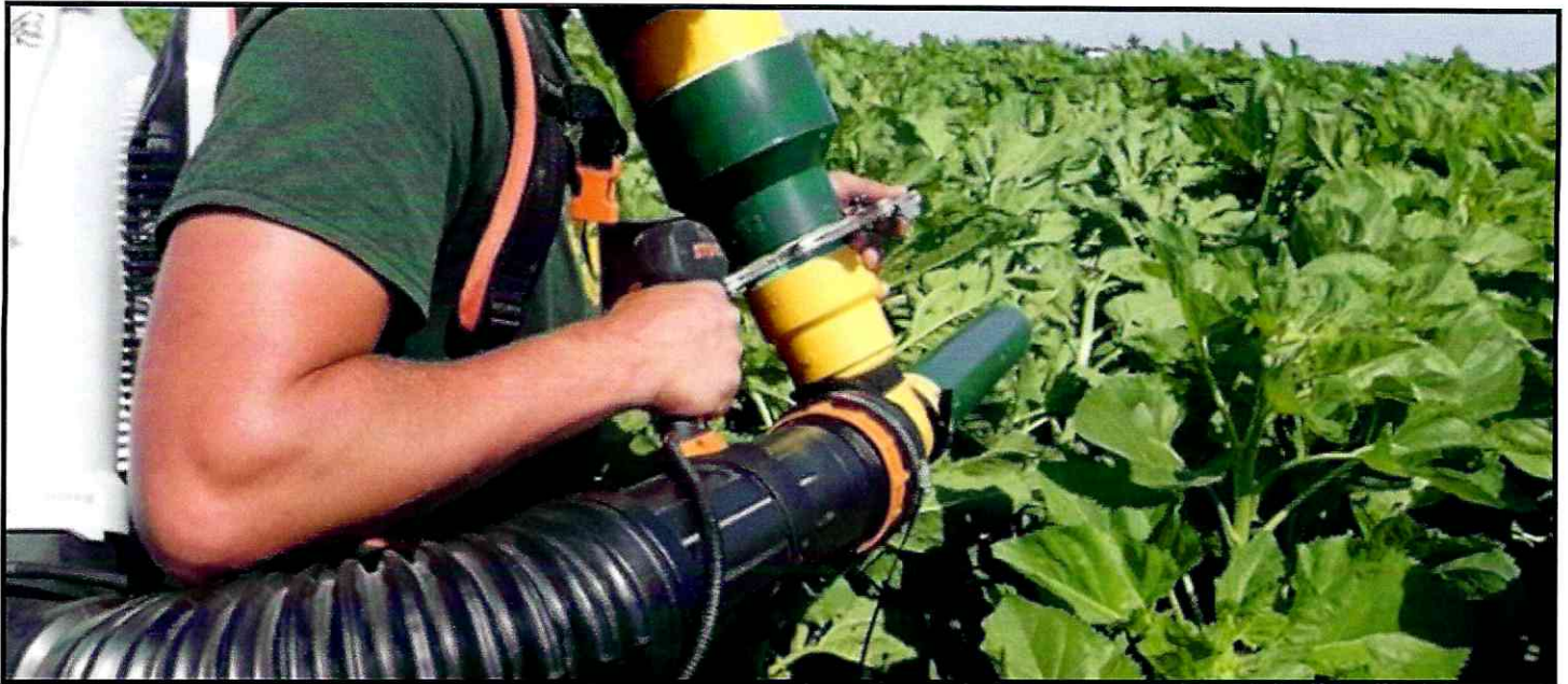
Application of simulated pea-size hail through prototype hail machine
