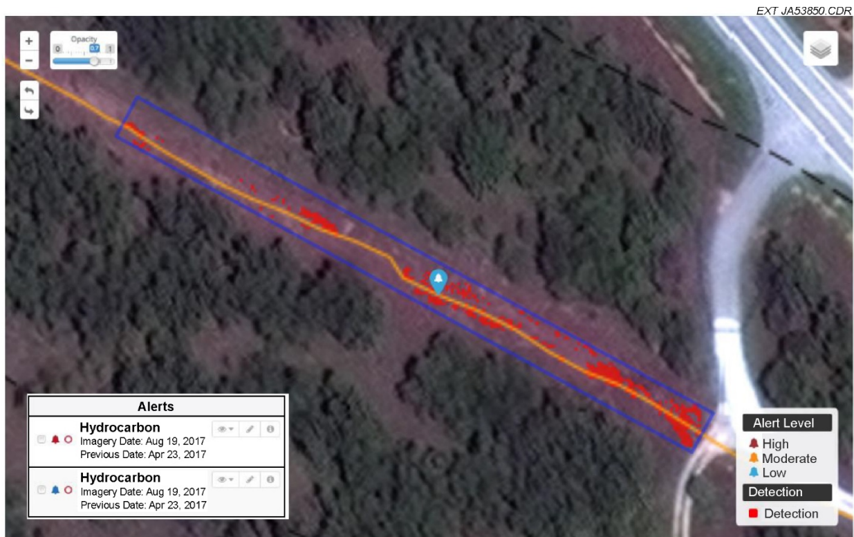
Figure 7. Identification of pipeline hydrocarbon spill by Satelytics (courtesy of Satelytics).
