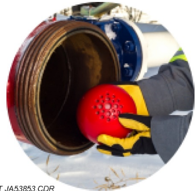
Figure 10. SmartBall in pipeline (courtesy of Pure Technologies).
