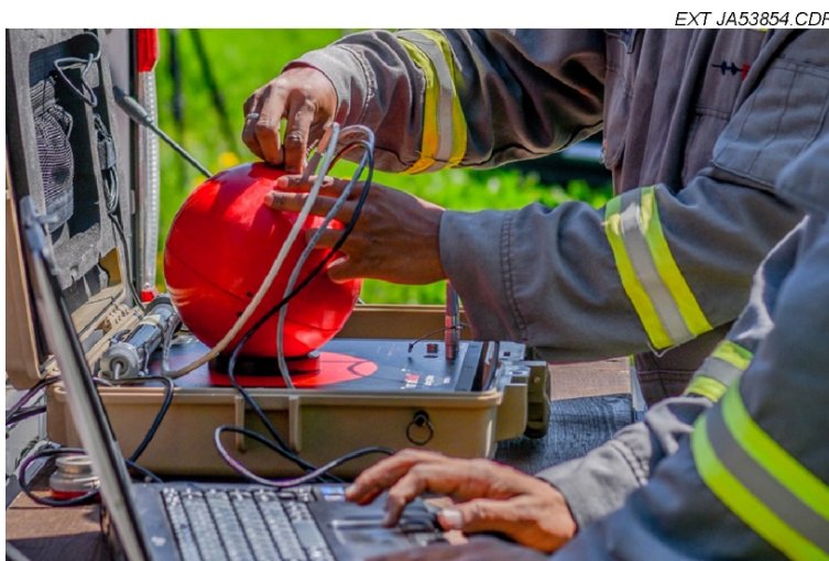
Figure 11. Technicians extracting data from SmartBall (courtesy of Pure Technologies).
