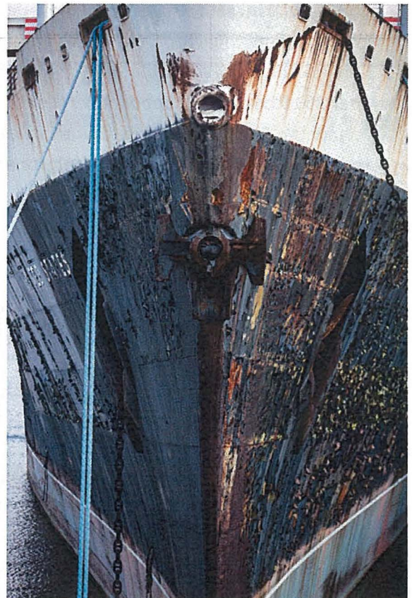
Corrosion on a Navy ship, National Geographic
