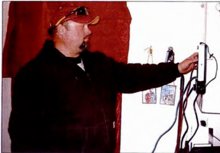
Bill Durwin with Community Action Partnership, standing in front of a door with a blower fan, set up to conduct a test to check for tightness of a FEMA home in southeast Minot Tuesday.
