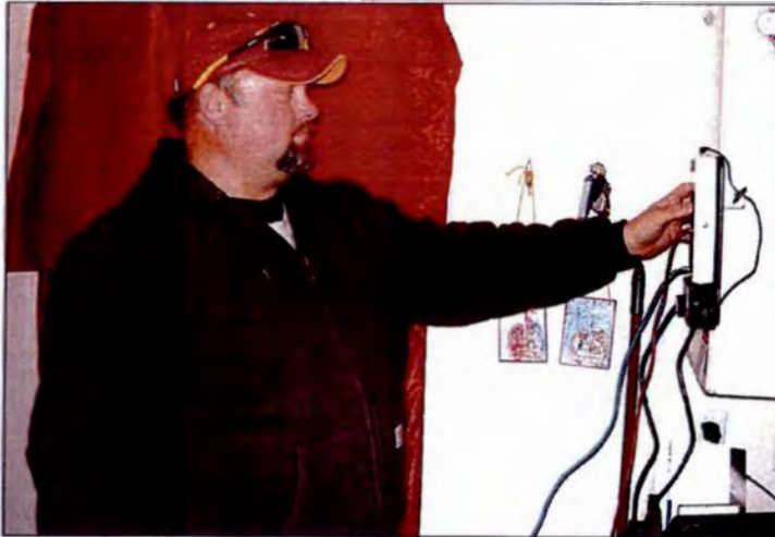
Bill Dunn with Community Action Partnership, standing in front of a door with a blower fan, sets up to conduct a test to check for tightness of a FEMA home in southeast Minot Tuesday.
