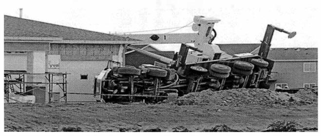
Truck Utilities said that the crane was not actually lifting anything when it went over, however the boom was almost fully extended. Construction workers at the scene did not say what caused the crane to tip over.
