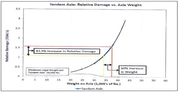
In fact, the relationship is exponential, which means that just a small increase in the axle load even for a short period of time exponentially increases the damage rate to the pavement.
