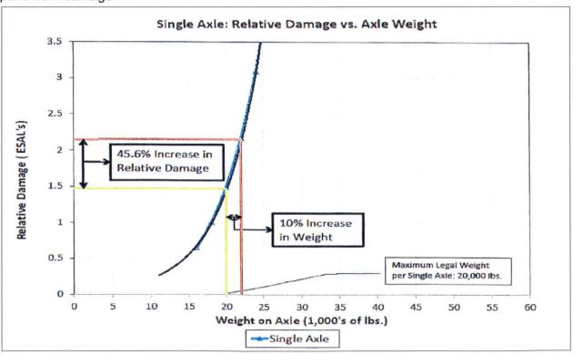
Every axle passing over a highway consumes a portion of the pavement's life. With each pass of a load, the pavement experiences forces that eventually lead to the deterioration of the pavement. Extensive testing has shown that the amount of pavement life consumed by heavy axles greatly exceeds the amount of life consumed by lighter axles.
