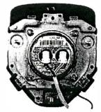
Airbag covers are engineered so that upon deployment, the cover splits along well designed tear seams. This creates a flap that allows the rapidly inflating bag to pass through the cover and create an air cushion without injuring the vehicle occupants. Counterfeits use poor quality molds and materials that do not open as designed.
