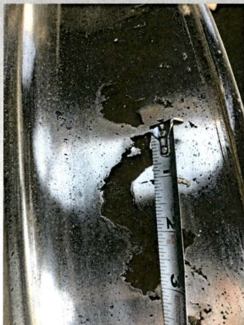
Defective Wheel Tread - Shelled
