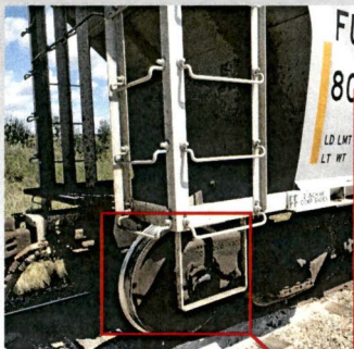
Defective Wheel Flange - Thin
