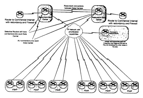
Although 12 PSAPs are indicated on the graphic, the two redundant data centers would be capable of serving the current 22 PSAPs.
