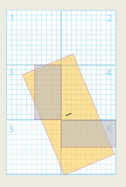
A turbine and access road will, on average, take about 2 or 3 acres out of agricultural production. If that turbine deploys an 80 meter rotor, and there are two opposing directions for seasonal prevailing winds, the turbulence from the turbine will involve 284.67 acres.
