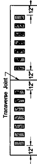
Discontinue rumble strip approx. 12" on both sides of PCC transverse joint
