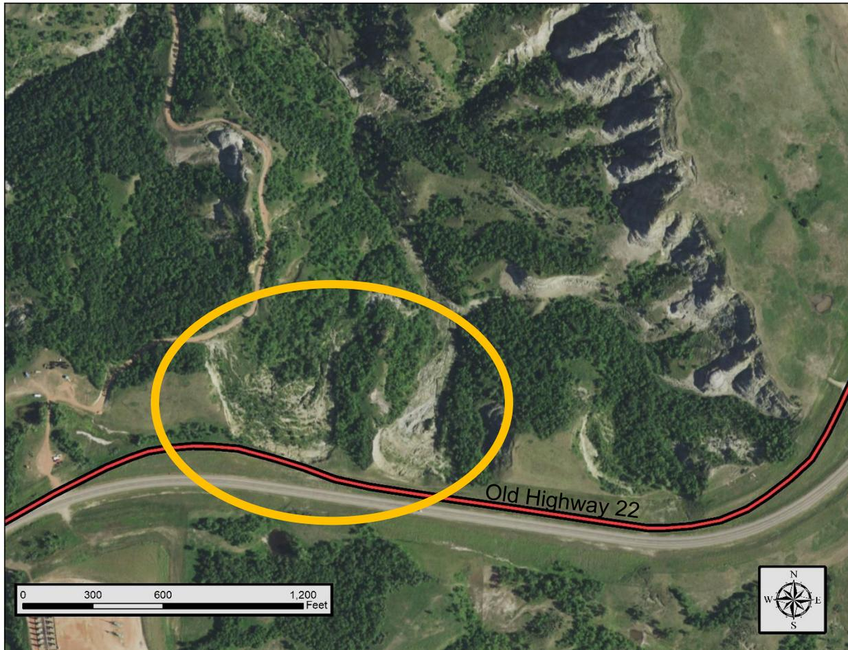
*A 2020 aerial photograph showing the present-day position of ND Highway 22 and the position of Hwy 22 in 1957 (in red). Encroaching landslides from the north forced the highway to be relocated to the south 100 feet or so in 2011.*
