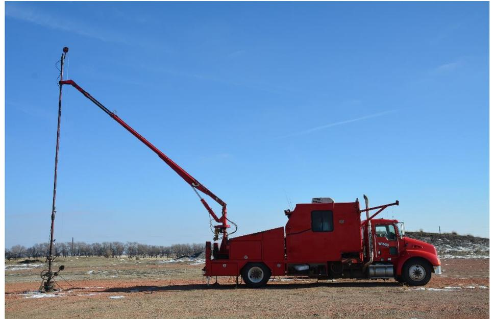
*Left: Black dots are wells we have temperature logged, green dots are wells that were temperature logged January 4-7, 2021, and the gray dots are TA'd wells that are potential candidates for logging. Right: Temperature probe being dropped into a TA'd well via a slick line truck.*
