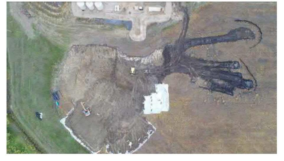
Photo #3 Stockpiling topsoil and excavated contaminated soil.
