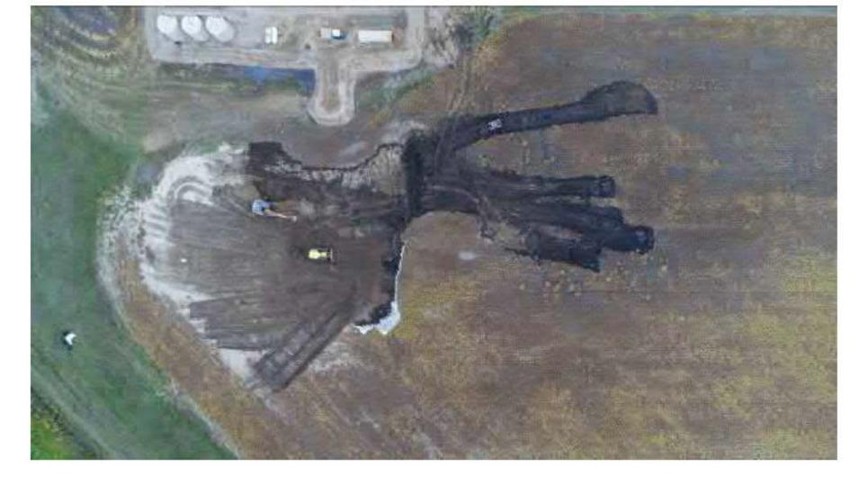
Photo #2 Initial earthwork and removal of topsoil.
