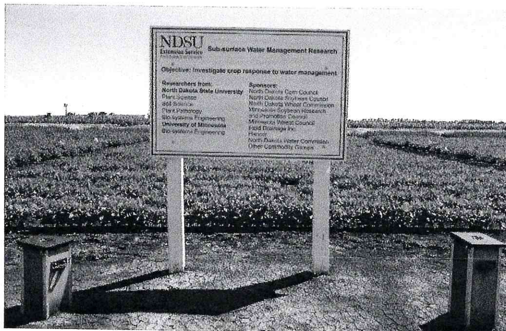
NDSU tile drainage research plots. Note the water level control boxes.
