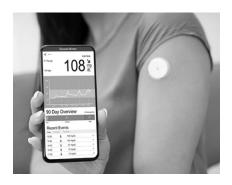
A sensor is inserted into the skin and held in place with an adhesive patch. Glucose readings are done every 5 minutes, continuously. A transmitter wirelessly sends readings to a device that displays blood glucose data. CGM systems use a dedicated monitor or a smartphone app.
