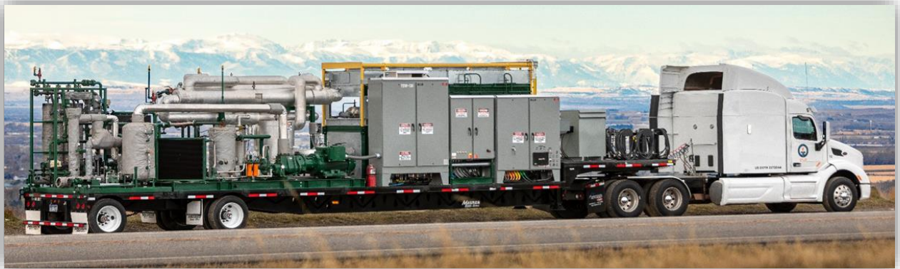
Figure 3: GTUITs Generation III TSW-1000 Wellsite Gas Processing System
