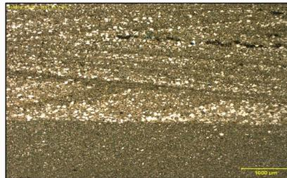
*Coarser grains and cross-bedding indicative of higher energy deposition in the upper half of a thin section from the Three Forks Formation at a depth of 9,785 feet in Williams County.*
