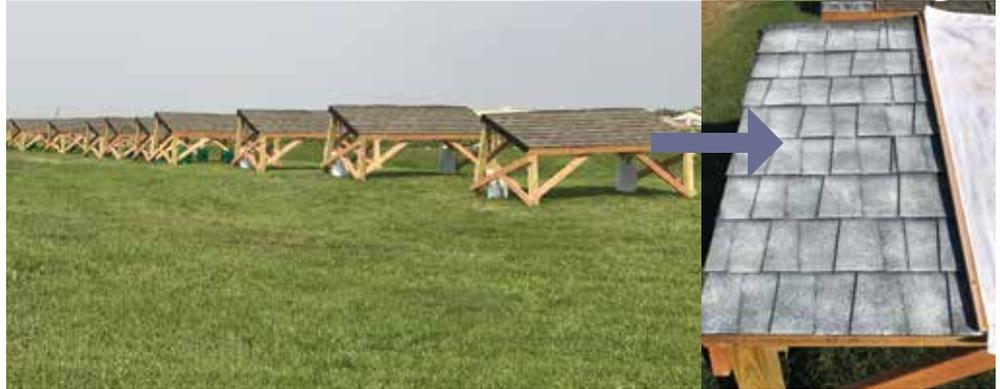
**Figure 1.** Ten test racks covered with 18-year-old shingles. Each rack was divided into four sections that were 2 x 4 ft. for treatment. Right-treated shingles before drying.
