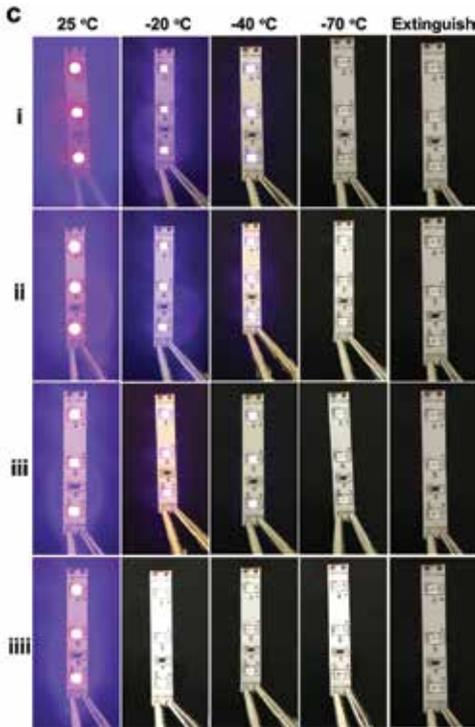
**Figure 1.** Visually demonstrated the conductivity of the hydrogels by using them to connect a circuit containing a light-emitting diode (LED).
