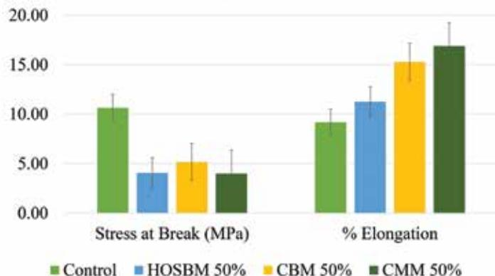
Effect of particle size of SBM-latex on mechanical performance of modified films
