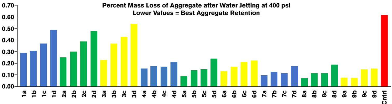
**Figure 2.** Water-jetting data with the untreated control. All treated shingles showed an improved aggregate adhesion. New shingles lost 0.34 wt. %.
