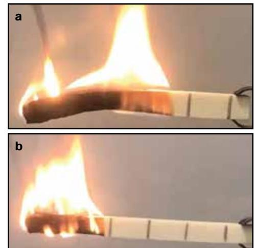
**Figure 1:** Horizontal burning test showing the rate of burning of soy-based PU foam samples. The above images show (a) sample with no flame retardant and (b) sample with 10 g of Cloisite 116A flame retardant. These pictures were taken after 50 seconds of burning. As seen, Cloisite 116A slows the spread of fire.
