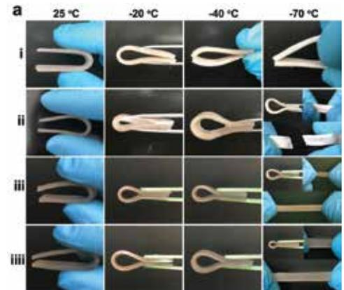
**Figure 2.** The flexibility and stretchability of the hydrogels demonstrated under different temperatures.
