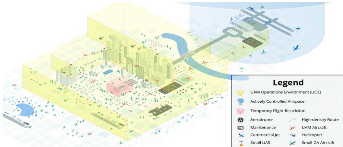
Figure 4. Isometric Operational View of a Representative UOE.
