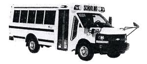
**Type B:** A Type "B" school bus is constructed utilizing a stripped chassis. The entrance door is behind the front wheels. This definition includes two classifications: **Type B-1**, with a GVWR of 10,000 pounds or less; and **Type B-2**, with a GVWR greater than 10,000 pounds.
