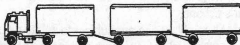
TRUCK-TRACTOR, SEMI TRAILER AND TWO TRAILERS OR TWO SEMI TRAILERS (TRIPLE BOTTOM) CONVERTED TO TRAILERS WITH CONVERTER DOLLIES
