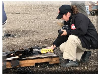
*Deputy Fire Marshal Jess Sinerius, using the PID to monitor for the presence of ignitable liquid vapors*
